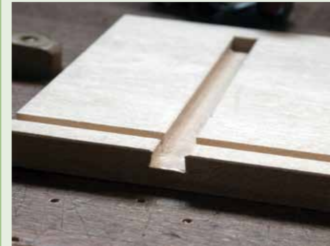
Drawer backs made with sliding dovetails require longer sides
