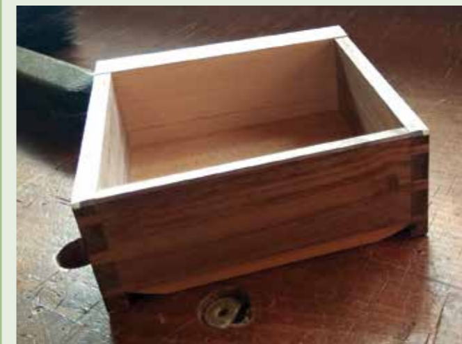
Regular drawers make better use of space but can be sloppy when made on a small scale
