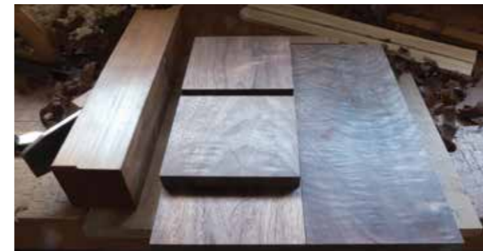
The pieces were all dimensioned on the shooting board
