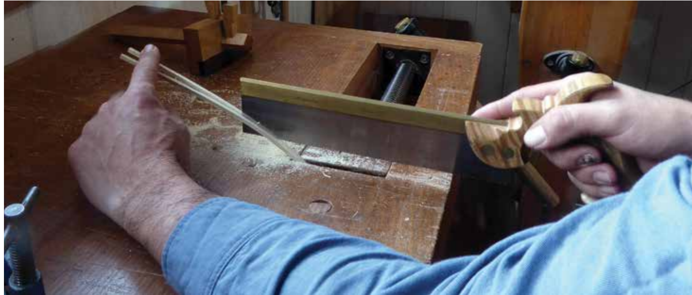
A dovetail saw is the perfect rip saw for small scale components
