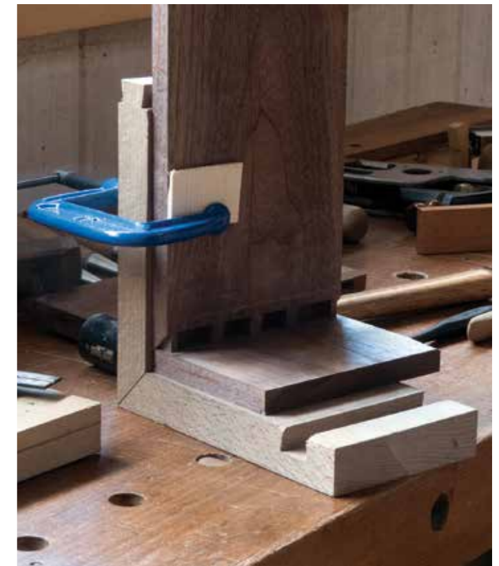
The pin board is clamped to the jig with the tail board below
