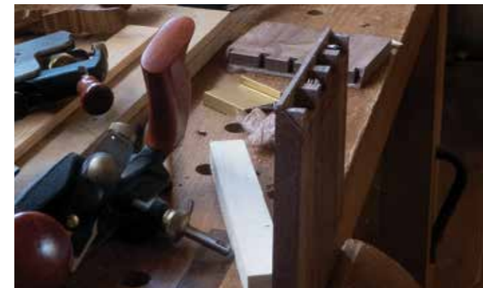
The pins are cut first and spaced so that transferring their positions is easier
