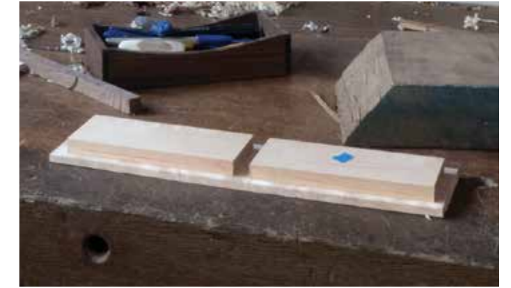
Laying out the drawer fronts on the veneer
