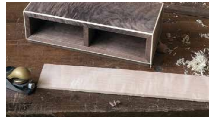
Ripple maple shop-made veneer for the drawer fronts
